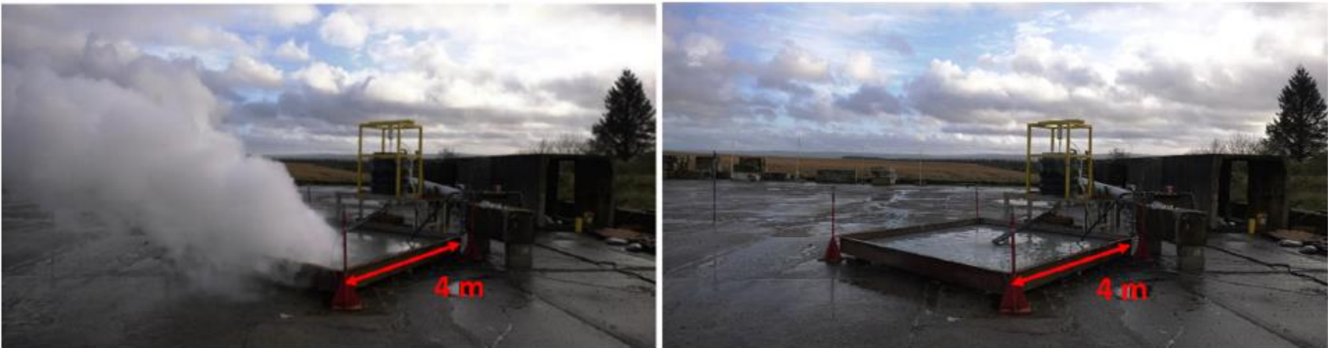
FIGURE 8 RS-1F unpressurized/cold ammonia spill on the water in bund with initial puff discharge for 18 s (left) and aqua ammonia pool after release (right). RS, Red Squirrel.
